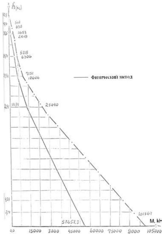
**Fig. 2. Distribution of bending moments along the height of the Kalon minaret.**
