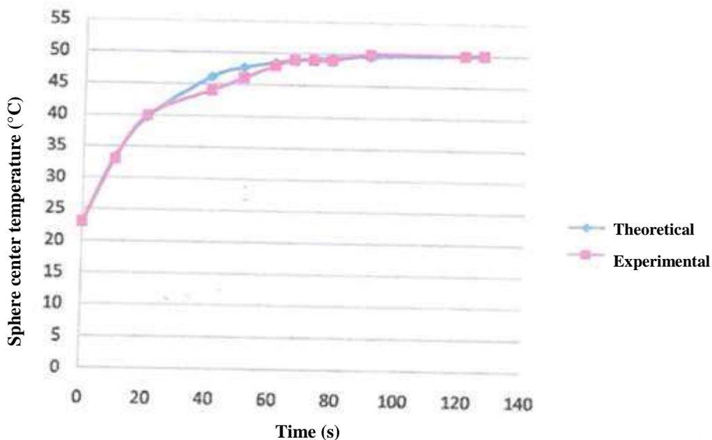
Graph 3.- Temperature profiles for aluminum sphere
