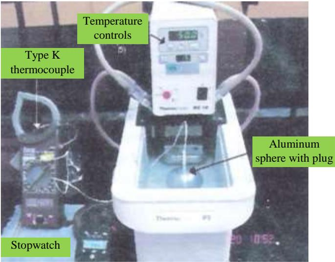
Figure 2.- Bath with aluminum sphere
