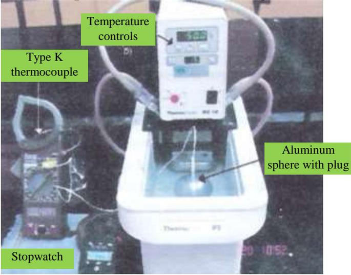
Figure 2.- Bath with aluminum sphere
