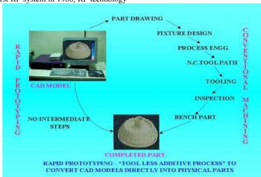
**Fig.1.RP in comparison to NC machining**
