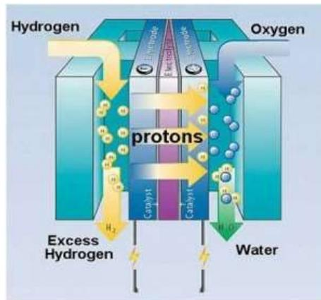
**Fig. 5. Working of a fuel cell**
