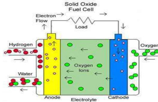
**Fig. 4 Drawing of a solid oxide cell.**
