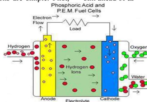
**Fig. 3 Drawing of how both phosphoric acid and PEM fuel cells operate.**
