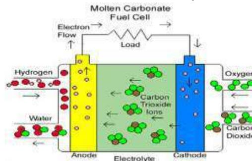
**Fig. 2 Drawing of a molten carbonate cell**
