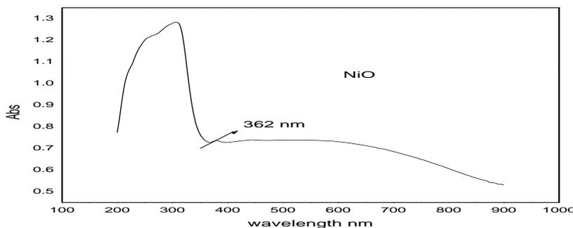
**Fig. 2 UV spectrum of NiO nanoparticles**
