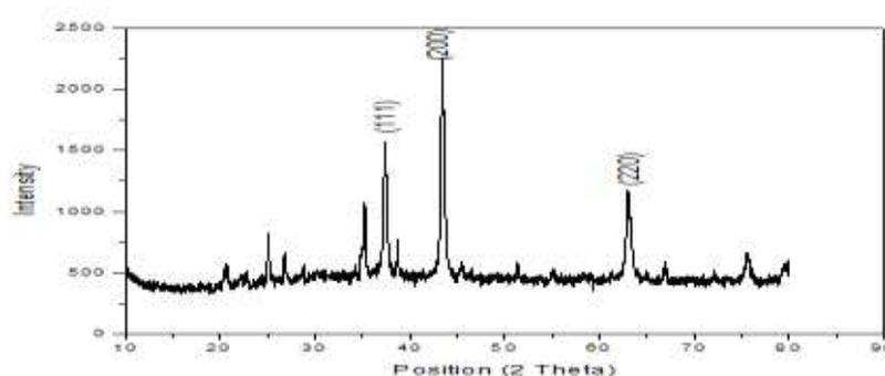
**Fig. 1 XRD - pattern of NiO nanoparticles**
