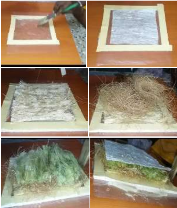
Composite preparation using HAND LAY-UP Method (GLASS-BANANA-COIR-SISAL-GLASS)
