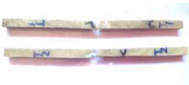
Tensile test specimen composite material
