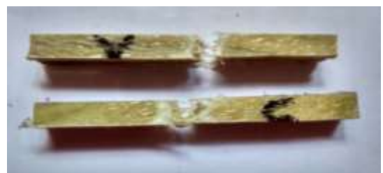
Impact test specimen composite material
