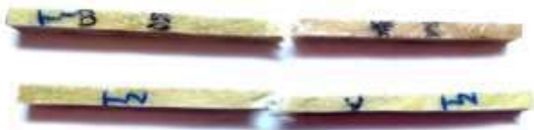
Flexural test specimen composite material
