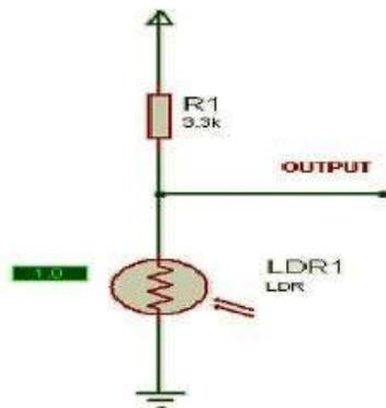
**Fig. 3 Light Intensity Sensor Circuit Diagram**
