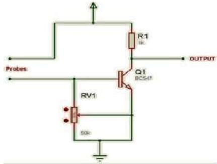
**Fig.2 Circuit diagram of the Soil Moisture Sensor**
