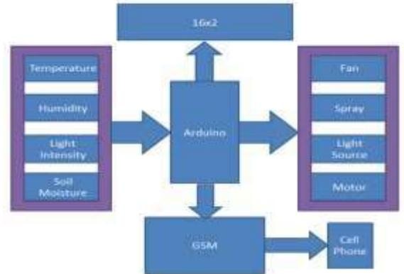
Fig. 6 Block Diagram of Proposed Remote Operating Station
