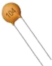
A  $0.1\mu\text{F}$  capacitor is placed in the circuit to connect the output from the piezo element to the input of the op-amp, also grounded on the op-amp side using a  $100\text{k}$  resistor. This acted as a DC decoupler and effectively lowered the comparator threshold required to detect vibration
