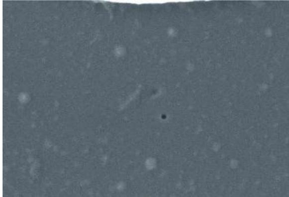
**Figure 12: E-beam quality assurance of 20 nm nanopore in 100 nm thick Si<sub>3</sub> N<sub>4</sub> membrane [4]**
