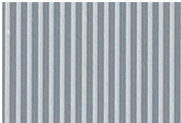
**Figure 3: SEM viewgraph of the etched grating [1]**
