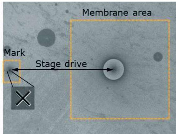
**Figure 6: verview SEM image of the silicon nitride membrane with active area including gold zone plate and reference mark on bulk sample for automatic positioning correction [3]**
