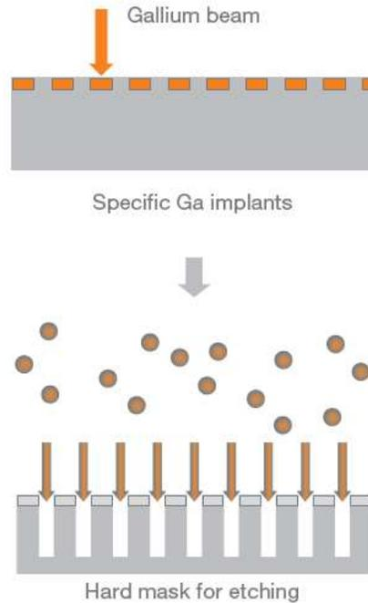
**Figure 2: Sketch of the functionalization process – after controlled Ga implantation trenches are etched into the substrate.**
