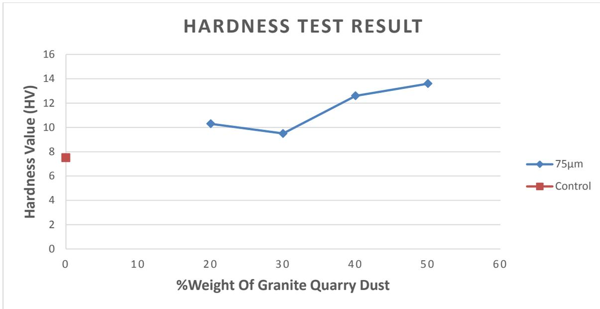
Fig. 3.1: Scatter diagram for Hardness Value against %weight of GrP
