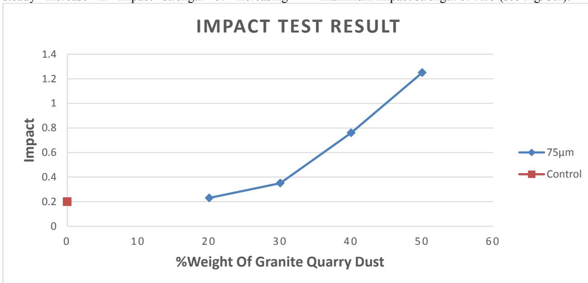
Fig. 3.2: A plot Impact test values against %wt of GrP
