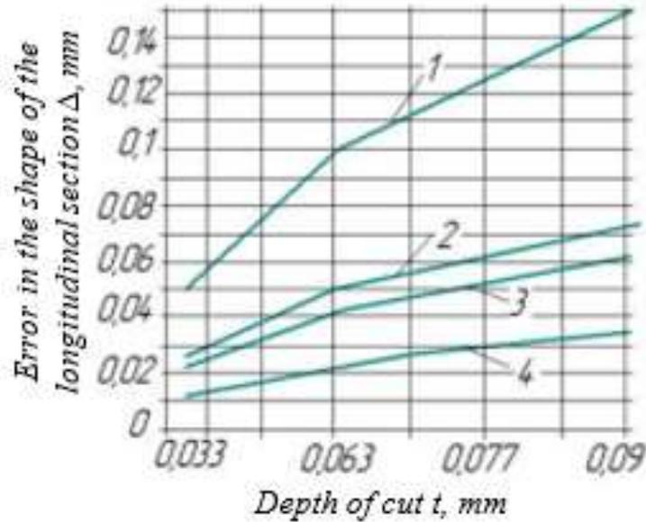
Fig. 2. Influence of the cutting depth on the accuracy of processing the screw surface
