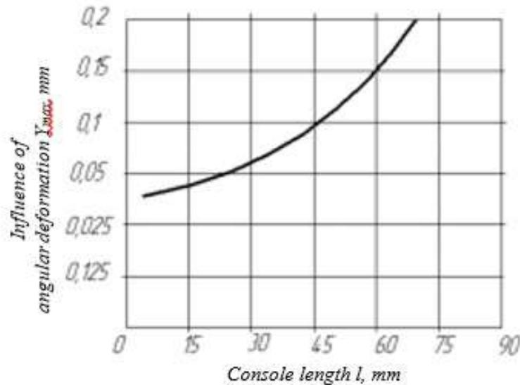
Fig. 3. Influence of the console length on the amount of elastic deformation of the work piece
