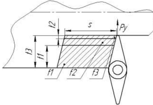
**Fig. 1.  $P_y$  dependence on the cutting depth  $t$ , mm and feed speed  $s$ , mm/rev.**
