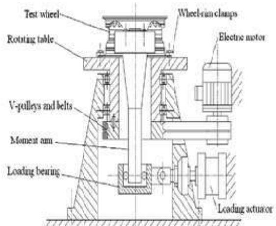
**Fig.6. Cornering Fatigue Test**
