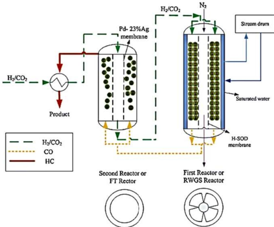
Figure 1. Synthesis gas production reactor
