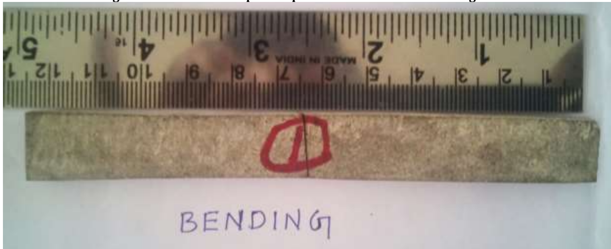
Fig 4 Cracked DRF composite specimen under Flexural strength test
