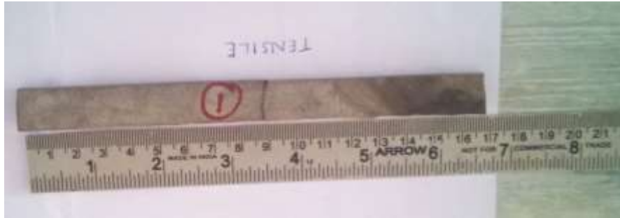
Fig 2 Cracked DRF composite specimen under Tensile strength test
