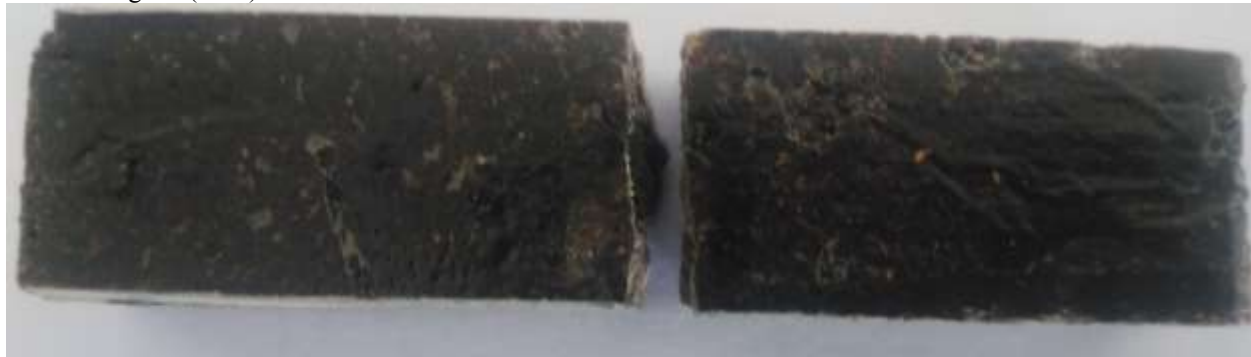
Fig 3 Cracked DRFG composite specimen under Flexural strength test
