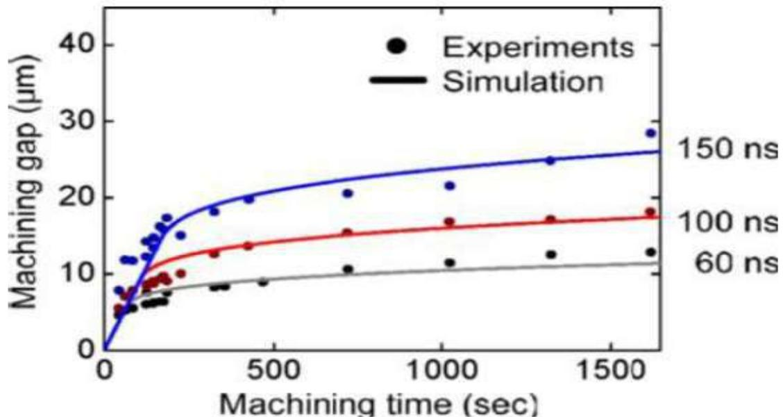
**Graph for machining time and machining gap**
