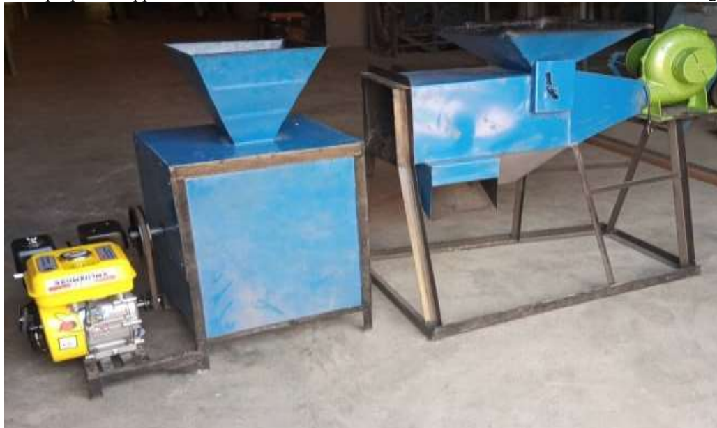
Figure 3 Showing the pictorial view of the assembled melon shelling machine
