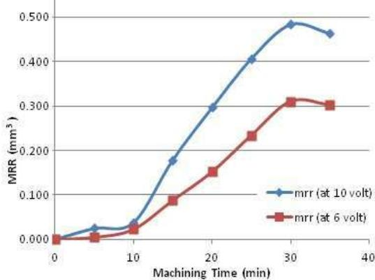
**Fig. 2 Graph between Material Removal V/S Machining Time**
