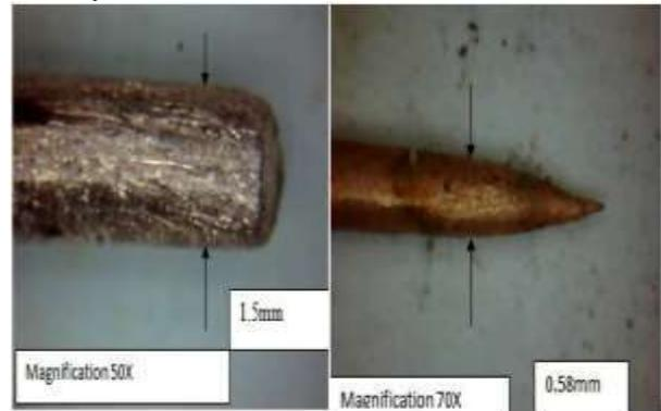
**Fig. 4 Tool fabrication at 6 volt 30gm/lit NaNO<sub>3</sub> electrolyte concentration (a) Anode copper wire before machining (b) Anode copper wire after machining**
