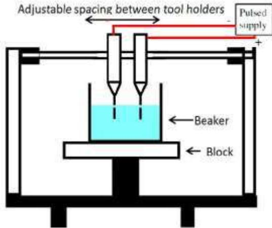
Fig. 1 ECMM Tool Fabrication Setup
