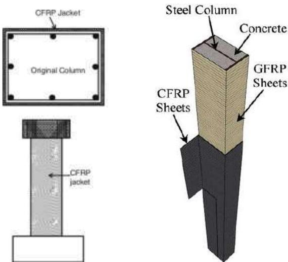
**Fig. 1. CFRP jacketing on column**
