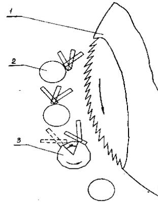
1-saw cylinder; 2-round fixed grates; 3-rotating multifaceted grate.
