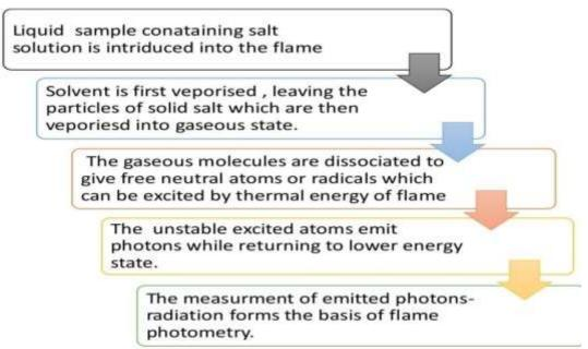
: Under constant and controlled conditions, the light intensity of the characteristic wavelength produced by each of the atoms is directly proportional to the number of atoms that are emitting energy, which in turn is directly proportional to concentration of the test sample.
