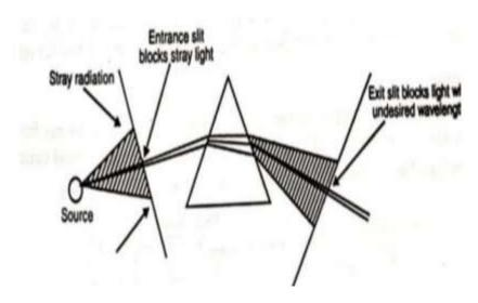
5) Monochromators: In simple models the Monochromators is the prism, but in expensive models, the gratings are. Prisms- Quartz is the material most commonly used for making prisms.
