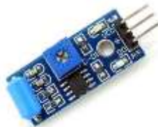
Figure: 03 – Visual representation of a typical vibration sensor.
