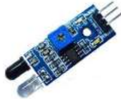
Figure: 02 – Visual representation of a typical IR sensor.
